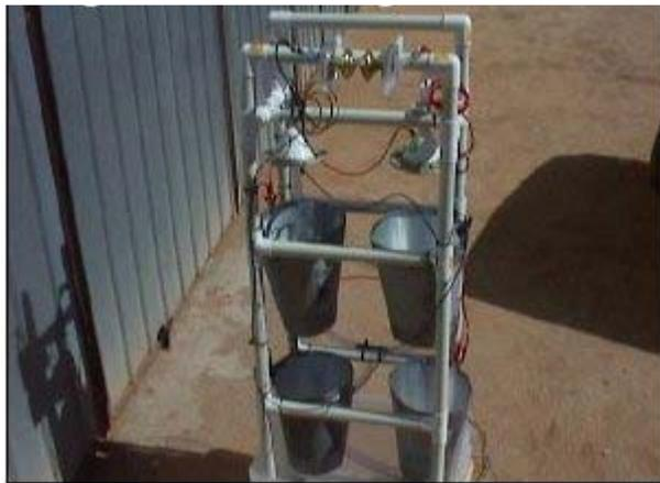
front view of author's unit notice the brass door knobs used as a spark gap.
