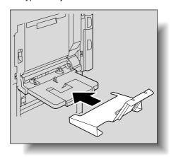
8 Erect the guide of the mounting kit.
