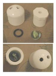
position. I have not fully tested the larger version. The outlet hole must be at least the same size as the water inlet hole to prevent the air from going out the wrong hole due to resistance. These need to be taken apart once a month and cleaned of the buildup in them. Picture link URL:
