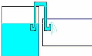
A J-Bend it is a tube bent like the letter “J” and used upside down. The long end is the drainage outlet end. The short end is where the water will enter and seal off the opening. Once the water level is high enough to cover the top of the upside down “J”, the siphon is started. These are used inside the container with the long end
